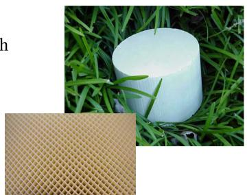
In addition, Cordierite is currently in mass production. It is commonly used in automotive catalytic converters and costs as little as 30 cents per cubic inch.
